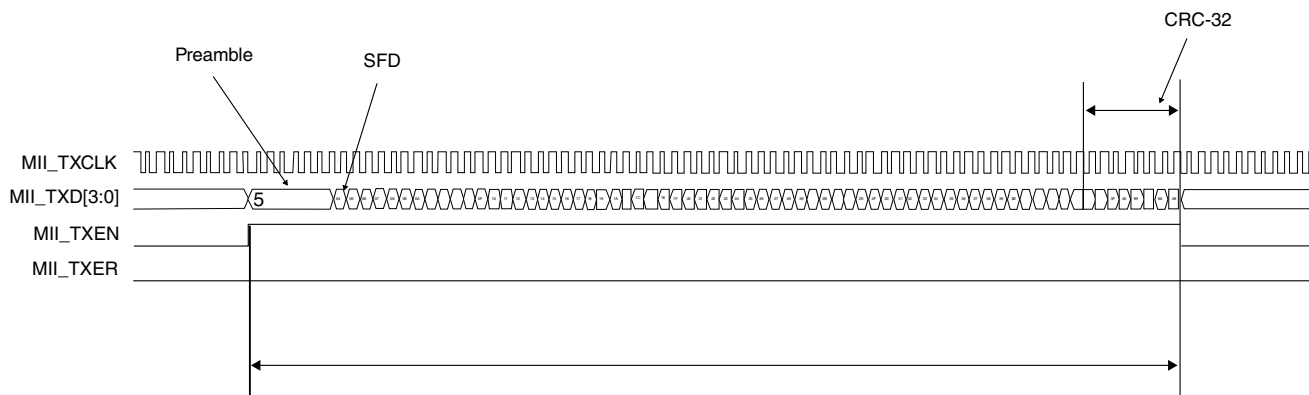
Figure 40-22. MII transmit operation
