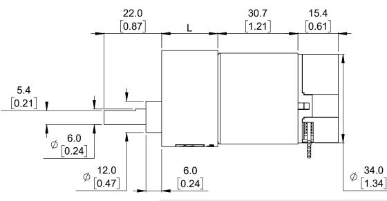
Threaded to a depth of 3.0 mm [0.12 in]; exceeding this depth can damage gears in the gearbox.
