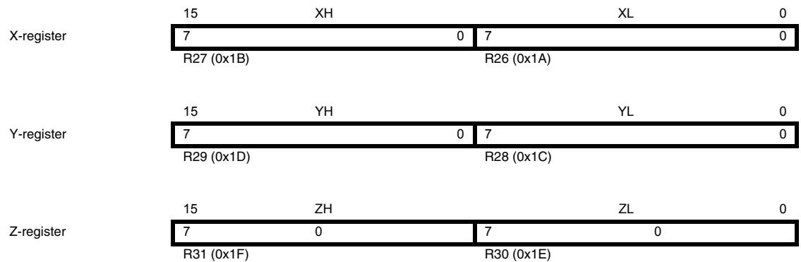
Figure 4-3. The X-, Y-, and Z-registers
