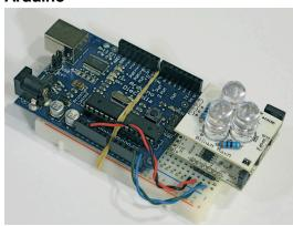
Photo 2.2.2 shows an example method of how to connect a MaxM to an Arduino. Note that unlike a BlinkM, a MaxM cannot be plugged directly into Arduino's Analog In pins 2,3,4,5 because the MaxM draws too much power.
