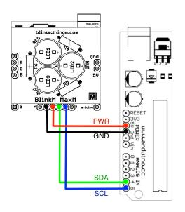
Photo 2.2.2: Connecting MaxM to Arduino
