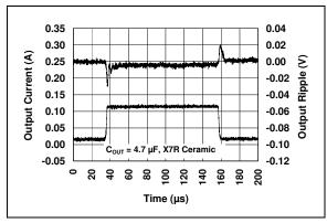
FIGURE 2-15: Load Transient Response.
