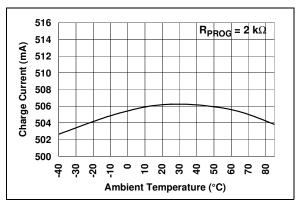
**FIGURE 2-8:** Charge Current  $(I_{OUT})$  vs. Ambient Temperature  $(T_A)$ .
