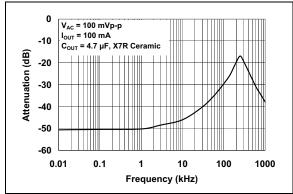
FIGURE 2-12: Power Supply Ripple Rejection (PSRR).
