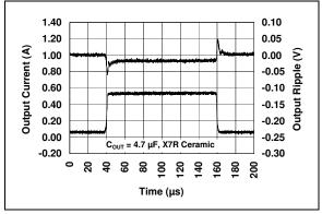
FIGURE 2-16: Load Transient Response.
