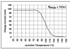
**FIGURE 2-9:** Charge Current  $(I_{OUT})$  vs. Junction Temperature  $(T_1)$ .
