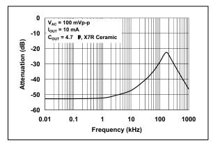
**FIGURE 2-11:** Power Supply Ripple Rejection (PSRR).
