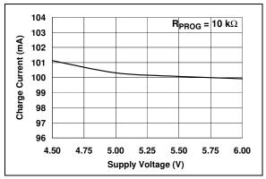
**FIGURE 2-5:** Charge Current ( $I_{OUT}$ ) vs. Supply Voltage ( $V_{DD}$ ).
