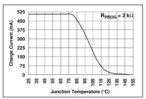
**FIGURE 2-10:** Charge Current  $(I_{OUT})$  vs. Junction Temperature  $(T_{.1})$ .
