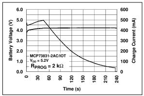
**FIGURE 2-18:** Complete Charge Cycle (1000 mAh Li-Ion Battery).
