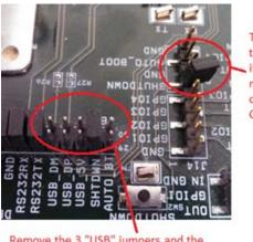
Remove the 3 "USB" jumpers and the AUTO\_BT jumper. These lines must be disconnected for the pre-production version of the Nano module to work properly. The SHUTDOWN line will turn off the Nano module if connected to GND. For normal operation, do not connect SHUTDOWN to GND.
