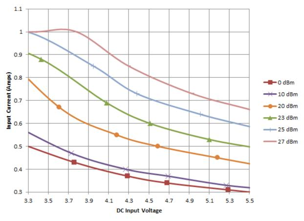
Current Draw vs. DC Voltage and RF Output Level
