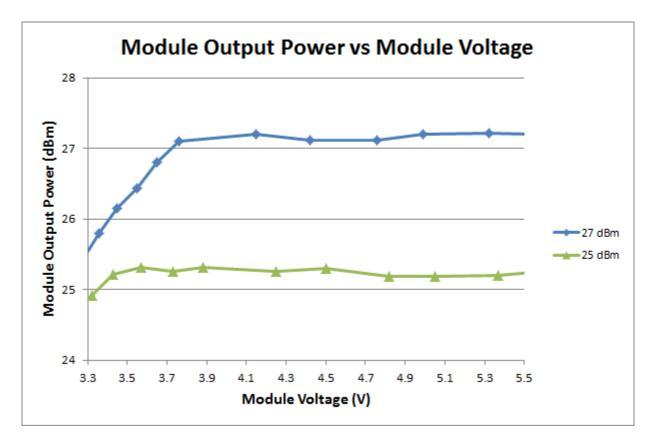
The power drawn by the module is fairly constant, rising slightly as the DC Input Voltage is lowered. Once the 1A input current limit is reached, the input power appears to
