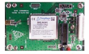
ThingMagic has created a Carrier Board for the ThingMagic Nano module, as an example of a host board for this module and to create an assembly that is compatible with the standard Development Kit main board. It has the size and dimensions of the M6e module (69 mm x 43 mm), and uses the same connector for power and control (Molex 53261-1571 - 1.25mm pin centers, 1 amp per pin rating. which mates with Molex housing p/n 51021-1500 with crimps p/n 63811-0300).
