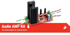
Your work room just got a little more musical! SparkFun's Audio Amp Kit is designed around a STA540 Power Amplifier. Once you have finished putting this kit together, you will have a fully-functioning two-channel amp, complete with a standby switch, volume control, and indicator LEDs. It's time to crank the volume up on your next project!
