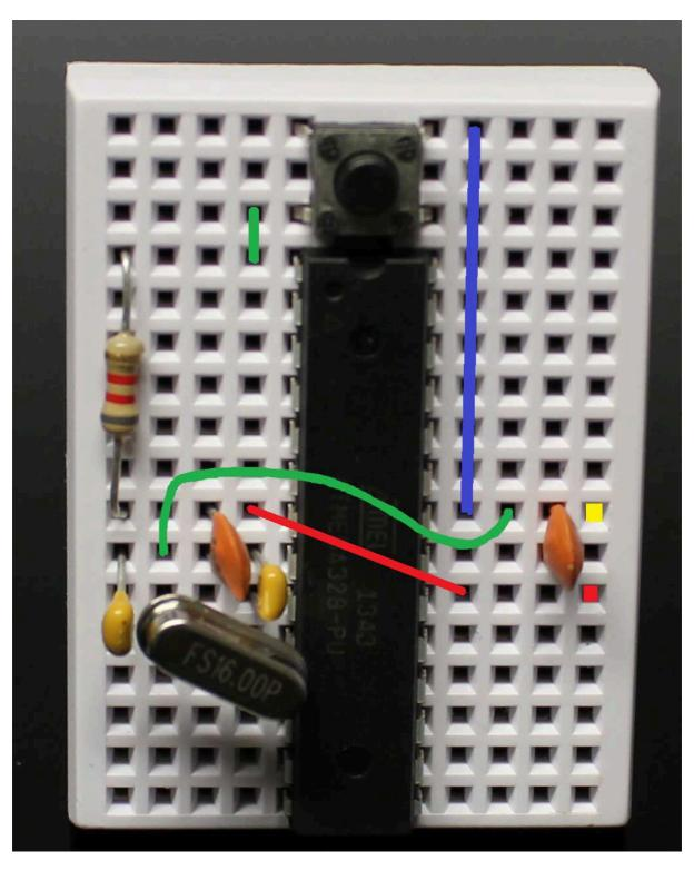
Place jumpers as shown above – the RED Square on the right is the POSITIVE Power connection and the YELLOW is the NEGATIVE (or Ground).
