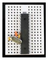
Mount the 16 Mhz crystal between pins 9 & 10
