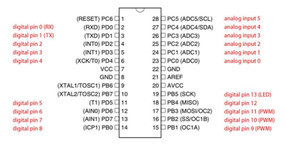
Here is the pin mapping for the ATMEGA328 chip to the equivalent Arduino pins.
