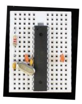
Connect the capacitor marked 103 between pins
