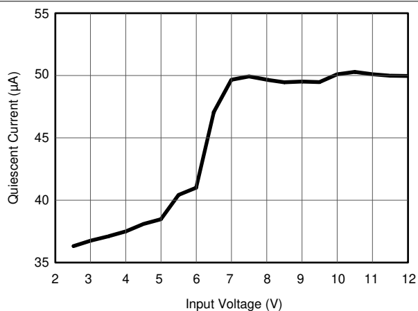
Figure 7-2. Quiescent Current vs Input Voltage
