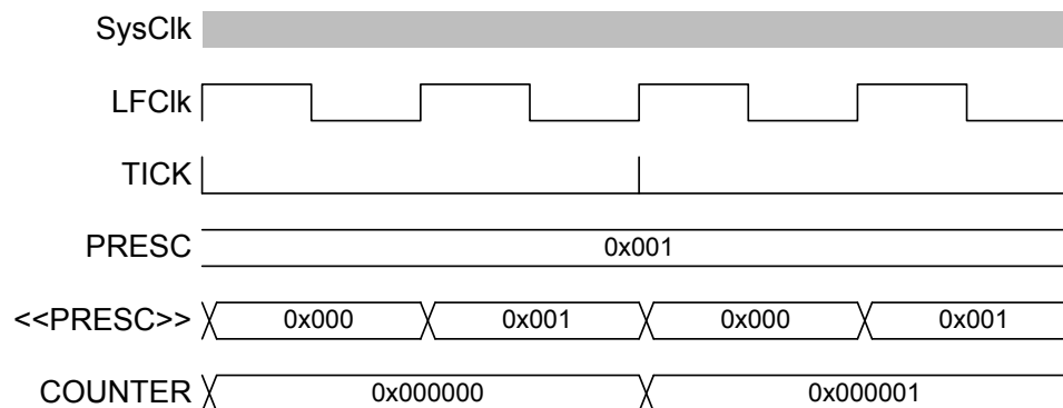
Figure 44: Timing diagram - COUNTER_PRESCALER_1
