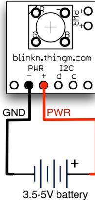
Photo 5.3: Battery Powered BlinkM
