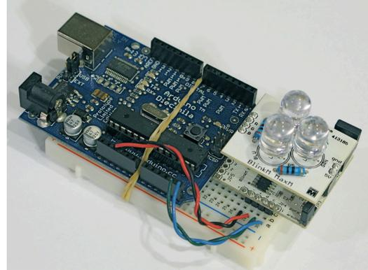
Photo 2.2.2 shows an example method of how to connect a MaxM to an Arduino. Note that unlike a BlinkM, a MaxM cannot be plugged directly into Arduino's Analog In pins 2,3,4,5 because the MaxM draws too much power.
