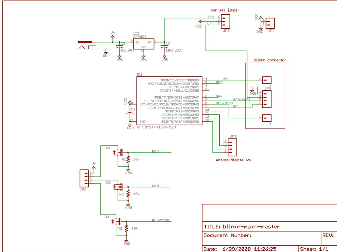
Figure 8.3: BlinkM MaxM “Blaster” LED board
