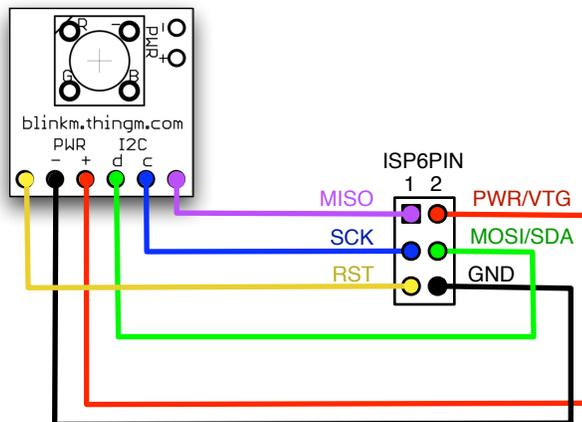
**Note:** most programmers do not supply power to the “VTG” (“PWR”) line, so power will need to be supplied to BlinkM in order to program it.
