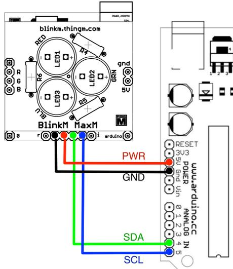
**Photo 2.2.2: Connecting MaxM to Arduino**
