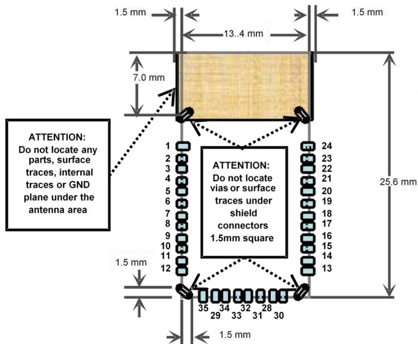
7. **Antenna Design.** The pattern from the rf\_out terminal pad should be designed with 50ohms impedance and traced with straight lines. (see diagram to the right) The rf\_out signal line should not run under or near the RN21 module. The GND plane should be on the side of the PCB which the module is mounted. The GND should be reinforced with through-hole connections and other means to stabilize the electric potential.
