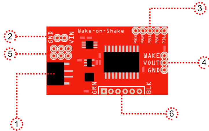
1. 2.0mm JST connection for power input: mates to SparkFun's single-cell LiPo batteries, or to SparkFun cable PRT-09914.
