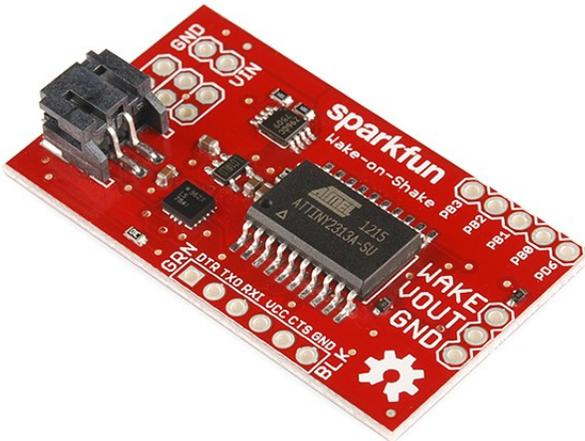
The Wake-on-Shake is intended to allow you to design a project which will remain inert for long periods of time (possibly up to several years, depending on the battery type used to power the project) until someone bumps, touches, or moves it. Its extremely low power consumption (<2uA @ 3.7V) means that, in most cases, aging related self-discharge of the battery is the limiting factor of the deployed lifespan.
