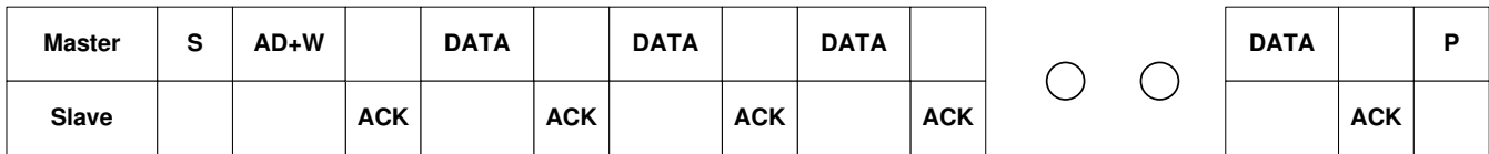
Figure 1-16: I 2 C write cycle
