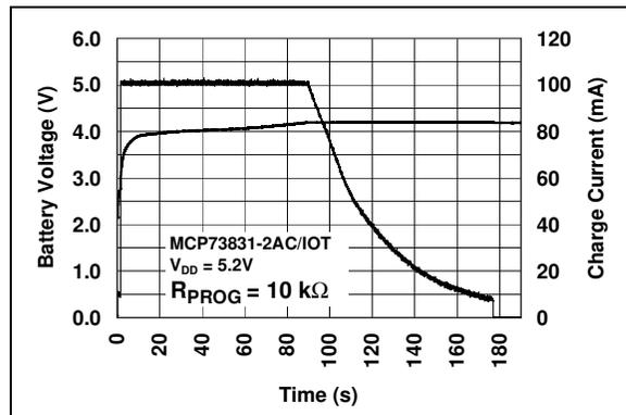
FIGURE 2-17: Complete Charge Cycle (180 mAh Li-Ion Battery).
