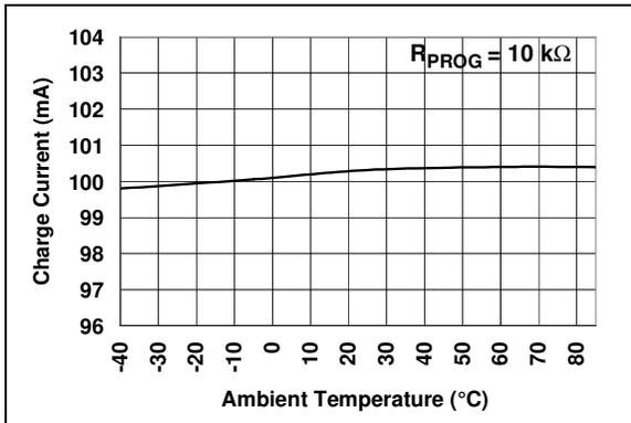
**FIGURE 2-7:** Charge Current ( $I_{OUT}$ ) vs. Ambient Temperature ( $T_A$ ).
